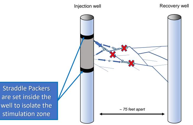
Diagrammatic cross-section through an injection and recovery well, showing schematic representation of fracture network. Not to scale.
