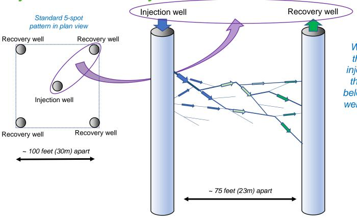
Weak acid is injected into the fractured rock via the injection well. It then moves through the fractured rock below ground to the recovery well where it is pumped back to surface, dissolving copper as it goes.
