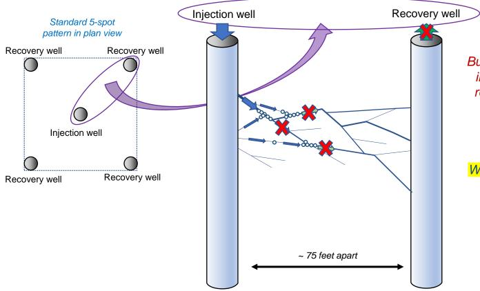
But gas bubbles form, collect in the fracture system and restrict flow. Flushing with water (or neutralized raffinate) removes the bubbles but is slow.
